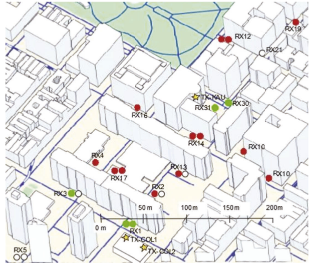
FIGURE 3: 3D building map of TX and RX locations around an urban area for 28 GHz measurements; stars indicate TX locations and dots indicate RX locations.
