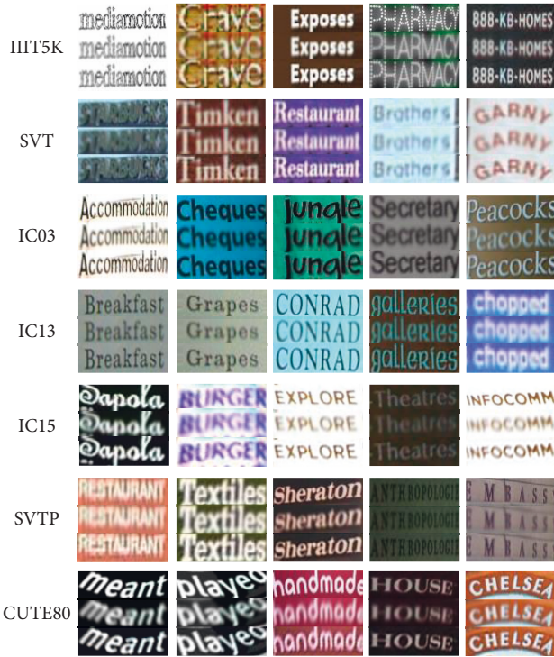
FIGURE 7: Performance of the adoption of Trans Conv2D in the super-resolution branch. In each image, from the top to bottom are the original image, blurred low-resolution image, and super-resolution image, respectively.
