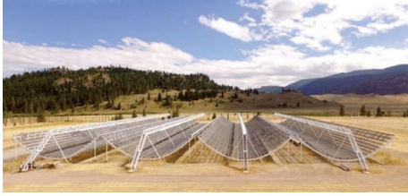
FIGURE 11: Canadian hydrogen intensity mapping experiment telescope ( https://nrc.canada.ca/en/research-development/nrc-facilities/dominion-radio-astrophysical-observatory-research-facility ).
