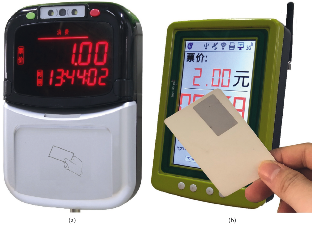
FIGURE 1: Two types of POS. (a) POS with up-down layout. (b) POS with antenna on LCD.
