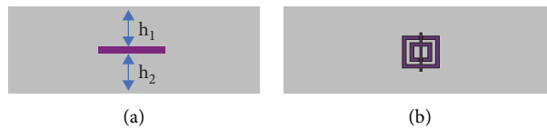
FIGURE 9: The substrate of the proposed metamaterial fractal antenna. (a) Front view. (b) Top view.
