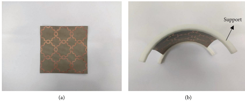
FIGURE 27: The fabricated prototype of the FSS. (a) Planar view. (b) Bending view.
