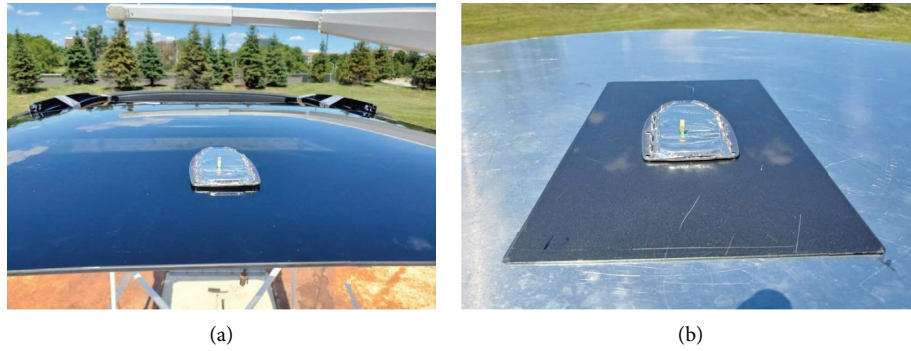
FIGURE 3: C-V2X monopole antenna when mounted on (a) vehicle’s glass roof and (b) 1-meter rounded metallic ground plane (GND).
