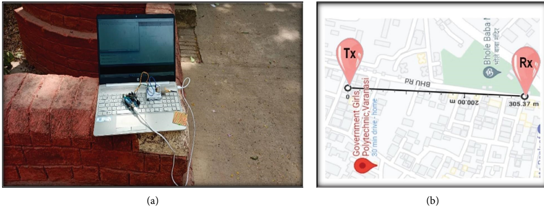
FIGURE 23: Third experiment-setup for in-building connectivity: (a) receiver set up and (b) map where the experiment (Tx-transmitter and Rx-receiver) performed.
