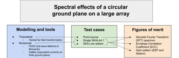
Flowchart of the Test Cases of this paper, as well as the Modelling and Tools used for computation and the Figures of Merit used for evaluation. Arrows and brackets show the resources used for one or more test cases
