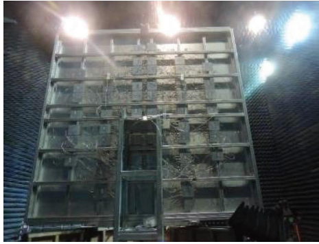
FIGURE 13: Back view of the receiving during testing antenna.
