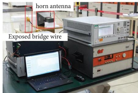
FIGURE 3: Test system of electromagnetic effect of EED under continuous wave.
