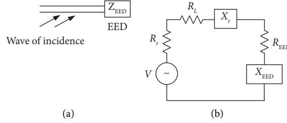
FIGURE 1: Equivalent circuit equivalent antenna and equivalent circuit of EED in the equilibrium mode. (a) Equivalent receiving antenna of EED in the equilibrium mode. (b) Equivalent circuit.
