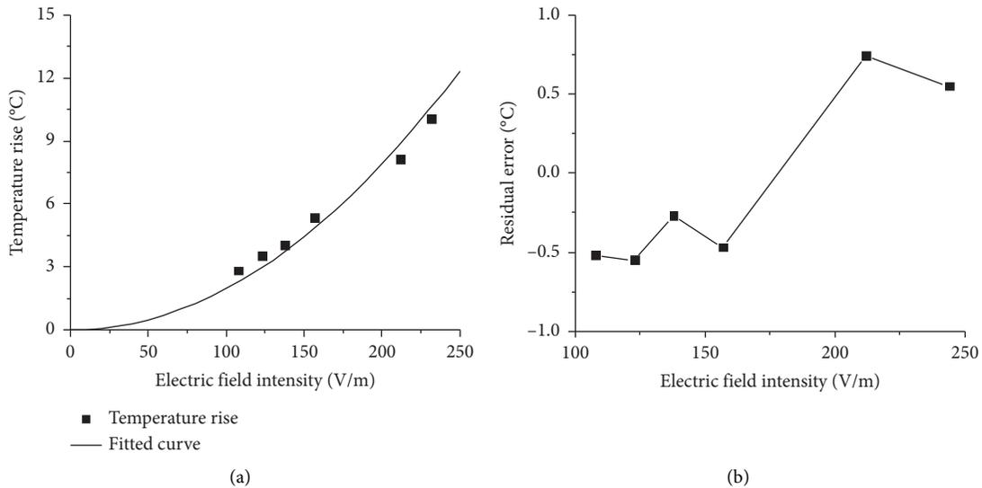
FIGURE 4: Bridge wire temperature rise fitting curve and fitting residual under RF continuous wave. (a) Fitting curve of bridge wire temperature rise. (b) Residual temperature rise error of bridge wire.
