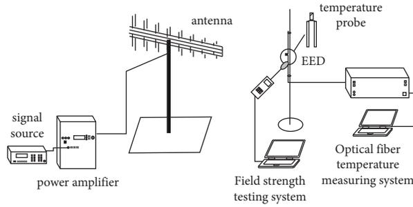
FIGURE 2: Test principle of electromagnetic effect of EED under continuous wave action.
