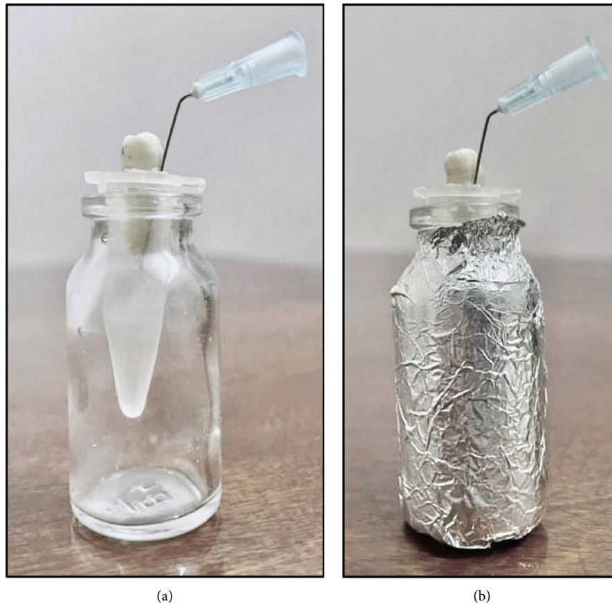
FIGURE 1: The experimental model used to evaluate debris extrusion (a, b) samples before and after the aluminum foil application.
