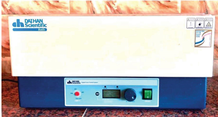
FIGURE 3: Digital water bath to mimic mouth temperature.
