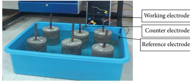
FIGURE 2: Setup of corrosion test.
