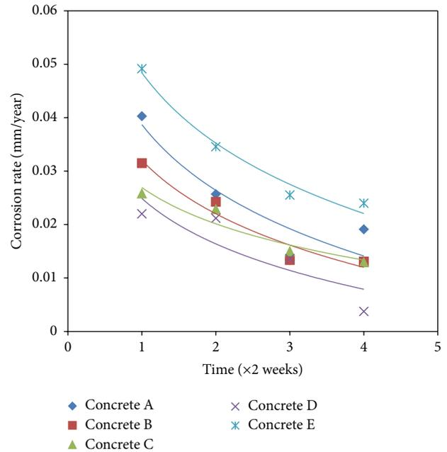
FIGURE 5: Corrosion rate of several types of concrete in 3.5% NaCl solution after immersion for 365 days.
