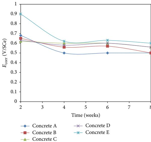
FIGURE 3: Effects of rebar on corrosion potential in 3.5% NaCl solution after immersion for 365 days.
