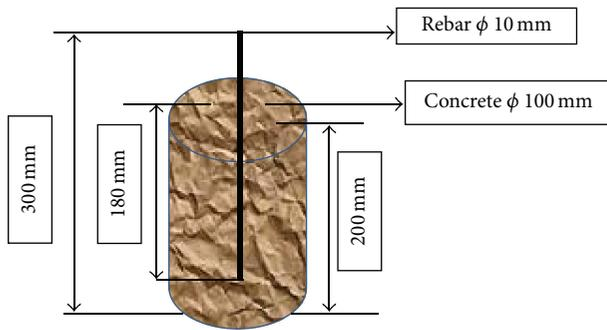
FIGURE 1: Experiment setup of the corrosion test.
