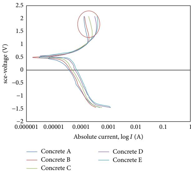
FIGURE 4: Polarization scan of rebar in 3.5% NaCl solution after immersion for 365 days.
