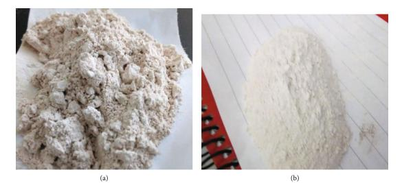
FIGURE 2: Photo images of (a) kaolin clay before and (b) after purification.
