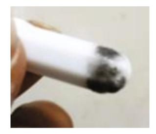
FIGURE 1: Magnetic beads with adsorbed impurities while purification of kaolin clay.
