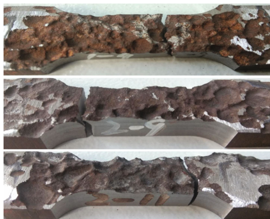
FIGURE 16: Surface morphology of fatigue test samples cut from bridge deck.
