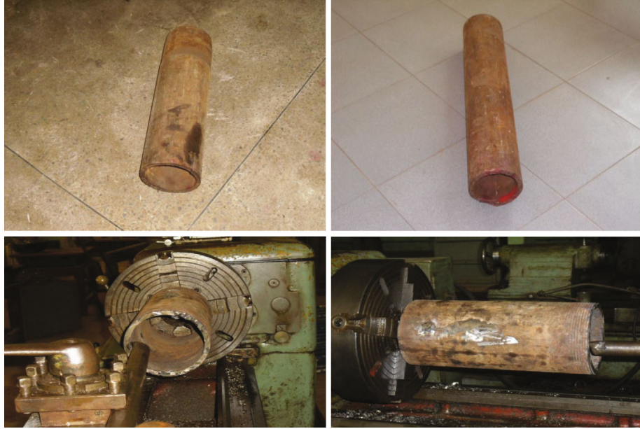
FIGURE 4: Machining of pipe using the lathe machine.
