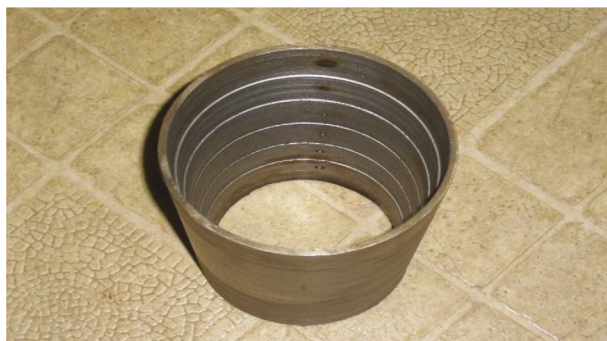
FIGURE 6: Interiorly machined pipe (test pipes).
