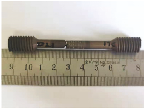
FIGURE 5: Appearance of fractured constant load test specimen.
