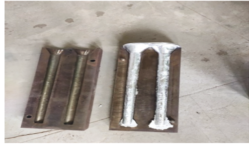
FIGURE 7: Die used in casting
