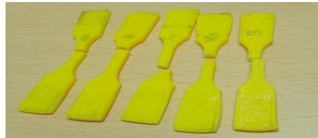
FIGURE 5: Failure tensile specimens (after tensile test).
