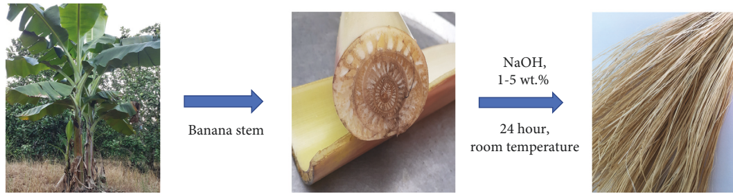
FIGURE 1: Retreatment process of Banana fiber (BF).
