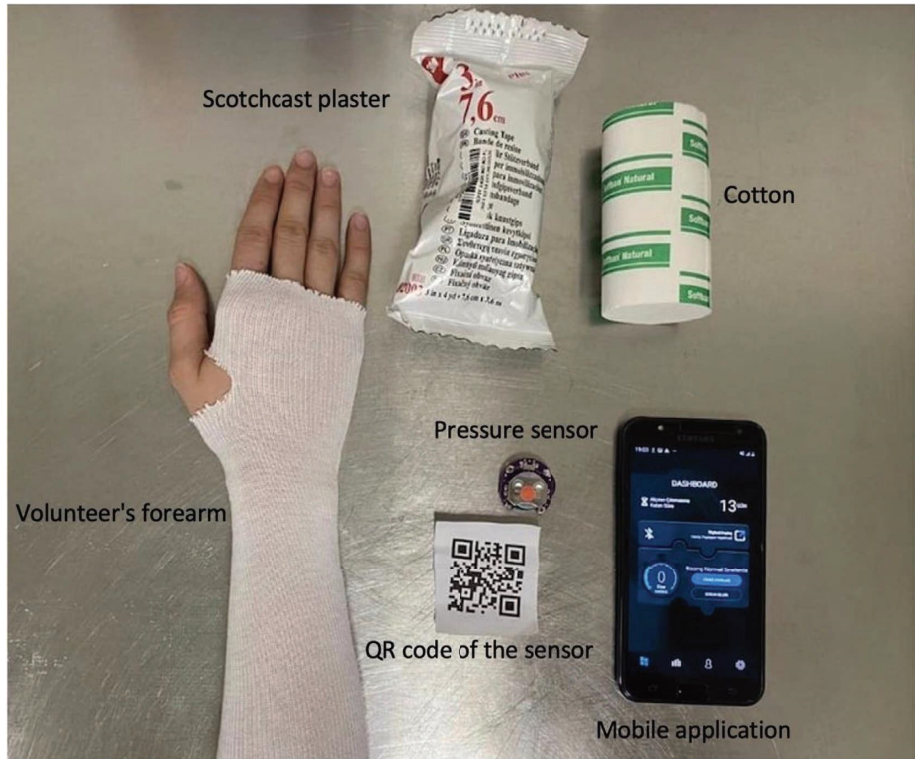
FIGURE 1: Materials required for skin-cast contact surface pressure measurement.
