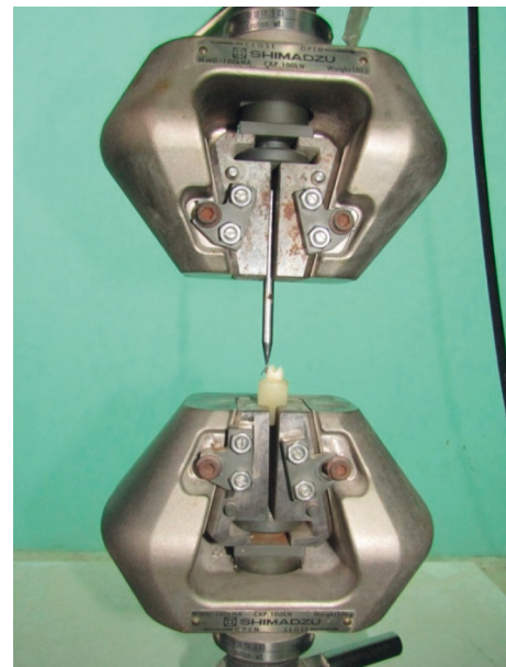
FIGURE 4: Close view of crosshead of the universal testing machine with sample in situ.
