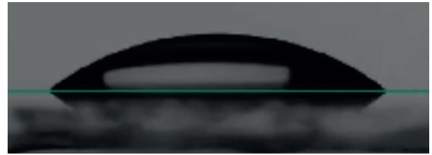
FIGURE 4: Baseline positioning using droplet reflection.
