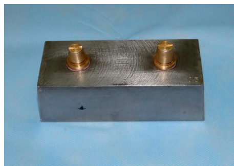
FIGURE 2: The main model used in this study to investigate the dimensional accuracy of the impression materials.
