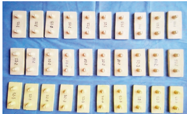
FIGURE 4: The casts prepared from two-stage Speedex impression at different times including 1 h, 24 h, and 14 days after impression (10 samples for each studied time).
