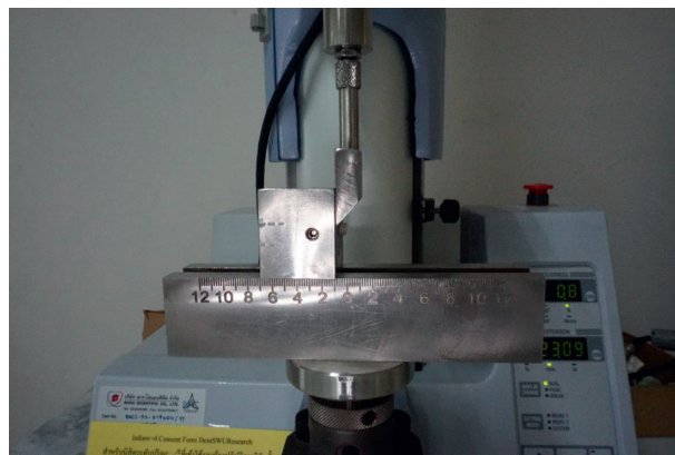
FIGURE 3: SBS test with a universal testing machine.
