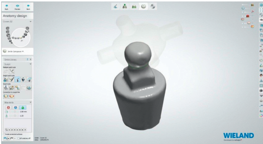
FIGURE 2: Scanned image of ball abutment analog.
