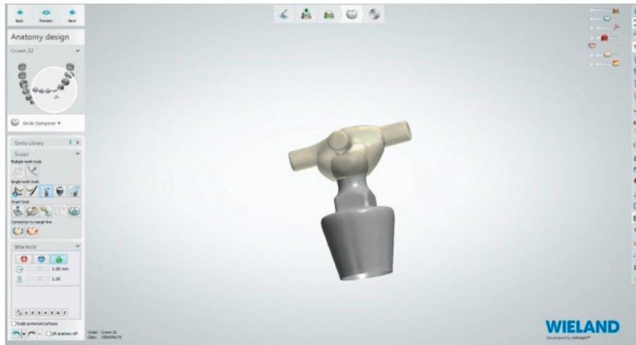
FIGURE 4: PEEK cap adapted to ball abutment.
