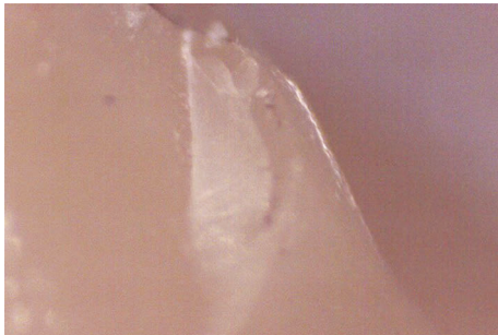
FIGURE 9: Stereomicroscopic images of the fractured crowns showing cohesive mode of failure at 35x magnification.
