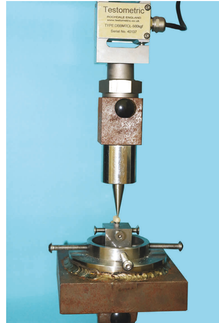
FIGURE 6: Metal tooth analog-crown-metal jig assembly mounted on universal testing machine (Testometric M350-5CT, Rochdale, United Kingdom).
