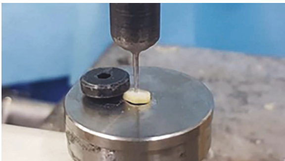
FIGURE 5: Push-out testing with a metal plunger.
