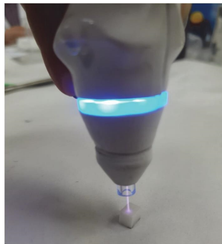
FIGURE 1: Nonthermal plasma treatment of zirconia samples.
