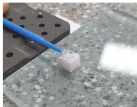
FIGURE 2: The jig designed for applying porcelain.
