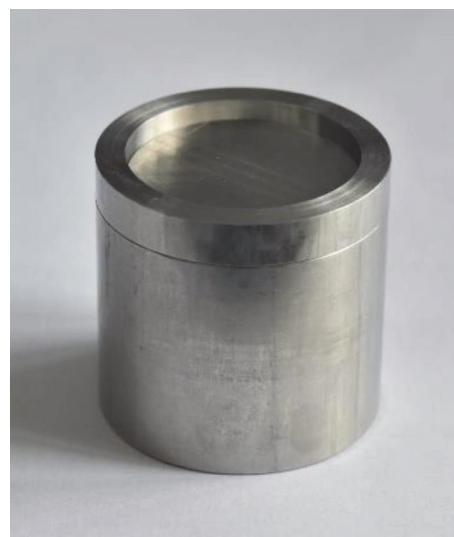
FIGURE 2: Stainless steel mold with ruled block.
