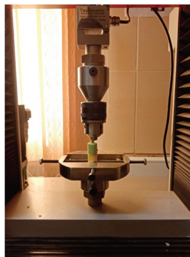
FIGURE 2: Pull-off test of samples with a universal testing machine.
