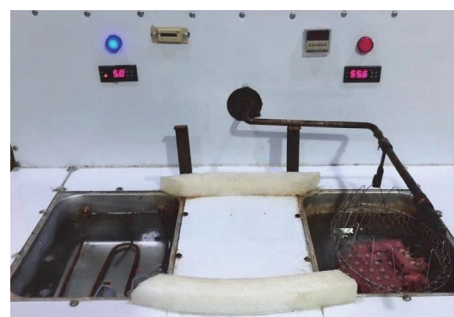
FIGURE 2: Thermocycling of 5,000 cycles between 5 and 55°C.
