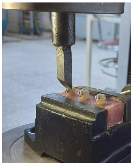
FIGURE 3: Fixation of the sample in the universal testing machine.
