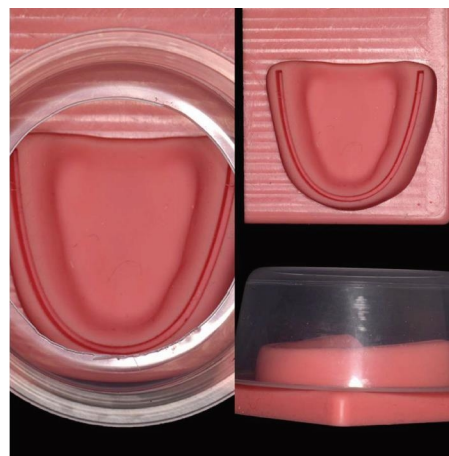
FIGURE 1: Flatbed and restricted models: left—top view of restricted version, bottom right—side view restricted model, and top right—unrestricted flatbed.
