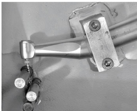
FIGURE 2: The instrument, while activated in a 60°, simulated root canal curvature at a water temperature of 37 \pm 0.5^\circ\text{C} .
