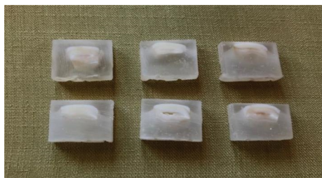
FIGURE 3: The embedded and cut samples in clear acrylic resin which were ready for the microhardness evaluations in three different depth of enamel.
