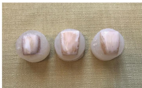
FIGURE 1: The mounted samples in acrylic resin after immersion in tea solution to simulate the discoloration in this study.
