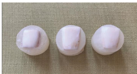
FIGURE 2: The mounted samples in acrylic resin after the different bleaching–remineralizing protocols.
