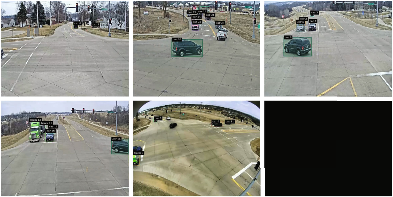
FIGURE 5: Result of the system with five video streams with the AI City Challenge dataset.
