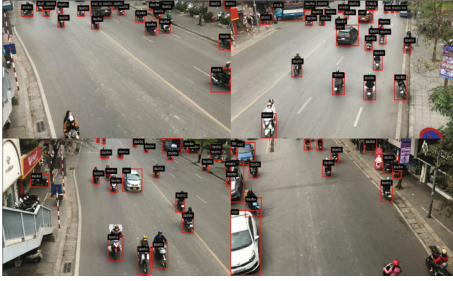
FIGURE 15: Results of running modules for detecting vehicles for four video streams.
