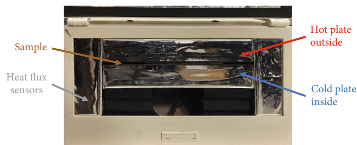
FIGURE 3: Heat flow meter to measure thermal conductivity.
