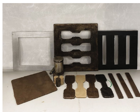
FIGURE 2: The four molds used in preparing the composite samples.
