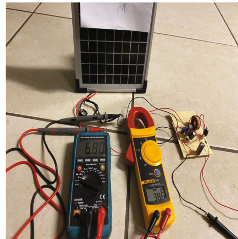
FIGURE 16: 50% solar output connection (photo taken during experimental setup by the authors).
