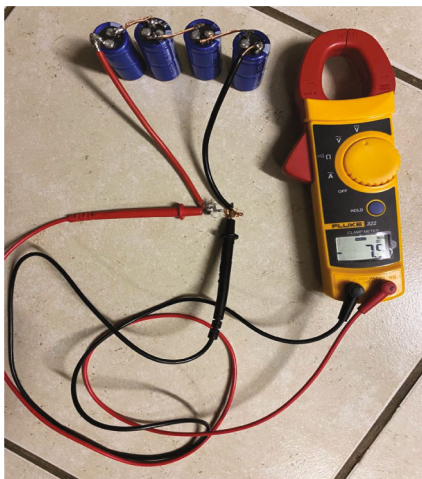
FIGURE 14: Output of SC after charging (photo taken during experimental setup by the authors).
