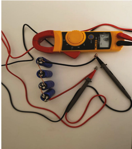
FIGURE 12: SC voltage before charging (photo taken during experimental setup by the authors).
