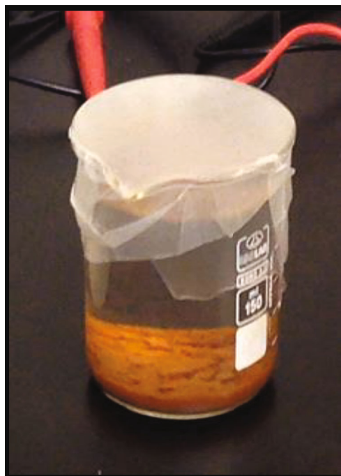
FIGURE 5: The corrosion deposits after only 7.5 minutes.
