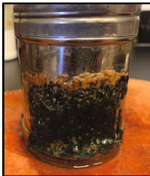
FIGURE 6: The corrosion effect on the positive electrode after only 7.5 minutes.
