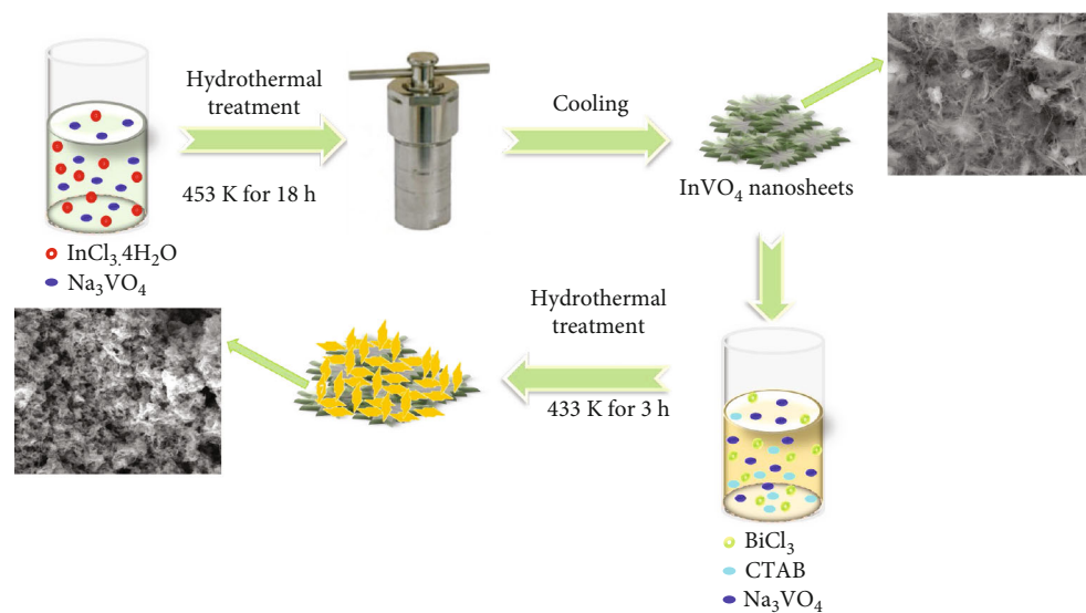
FIGURE 1: Schematic illustration for the formation of IVO/BVO heterojunction nanocomposites.
