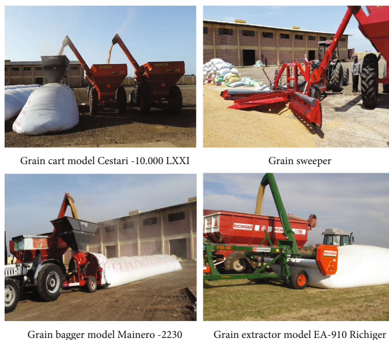
FIGURE 2: Machinery used for silo bag processing.
