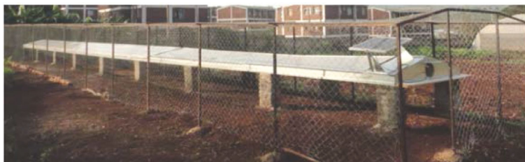
FIGURE 1: Real picture and schematic diagram showing details of solar tunnel drier used for the study and the three drying zones classified according to temperature and RH variation along the drier from absorber to exit end.
