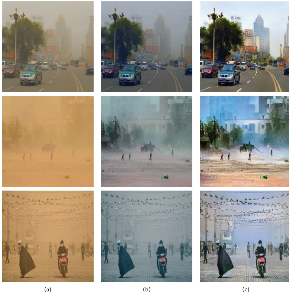
FIGURE 13: Two-step effect images of our method: (a) sand-dust images, (b) results of color correction, and (c) results of detail refinement network.
