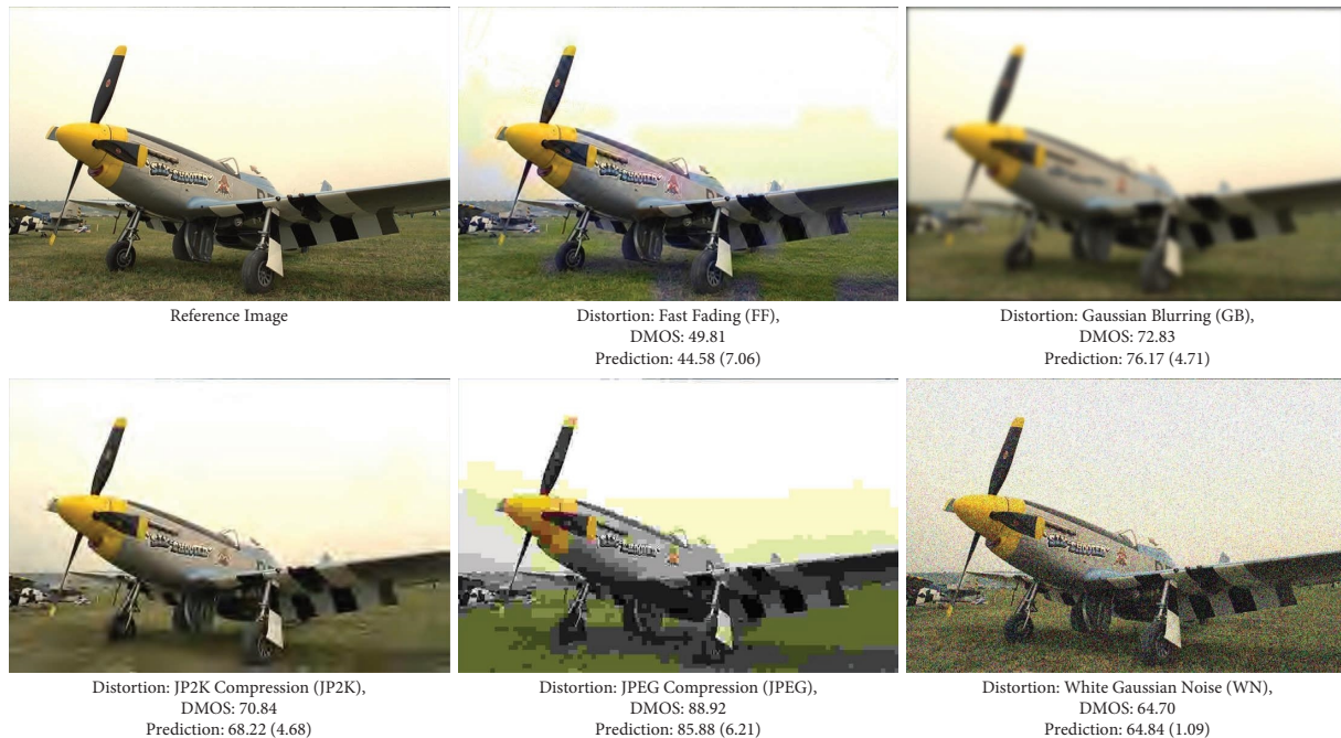
FIGURE 5: Scoring results of distorted images from LIVE. Image in the left top corner is the pristine image, and other five ones correspond to distortion types FF, GB, HP2K, JPEG, and WN. Values in parentheses behind the predicted score are standard deviations.
