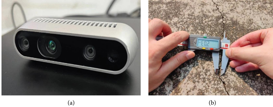
FIGURE 12: Equipment used for crack identification and measurement: (a) depth camera and (b) electronic Vernier caliper.
