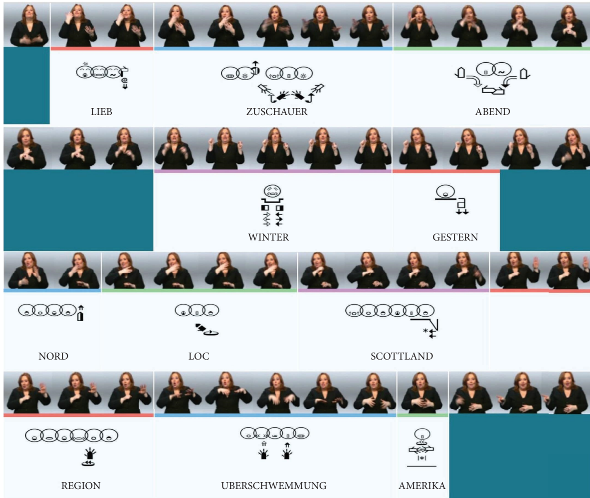
FIGURE 4: The FSC2 keyframe extraction algorithm: generated keyframes. The sentence “LIEB ZUSCHAUER ABEND WINTER GESTERN loc-NORD SCHOTTLAND loc-REGION UEBERSCHWEMMUNG AMERIKA” was condensed from 176 frames to 48 keyframes. The signwriting rendition is shown beneath each word.
