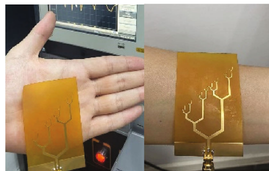
FIGURE 10: S11 schematic representation of the antenna placed on the middle of the forearm and palm during the test.
