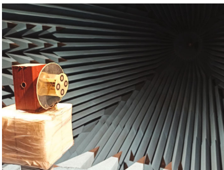
FIGURE 22: Photograph of the fabricated prototype of the proposed antenna and test setup.
