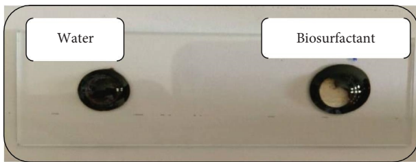
FIGURE 2: Drop collapse assay. Biosurfactant collapsed the hydrocarbon drop, while water was repelled from the hydrophobic surface.
