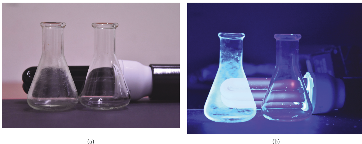
FIGURE 4: Two common laboratory flasks in natural light (above). The same flasks under a Wood's lamp light (below). The flask on the left is painted with 10% NPh2-PS blend.
